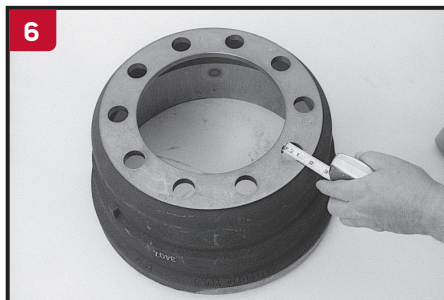
Number, size, and location of bolt holes
