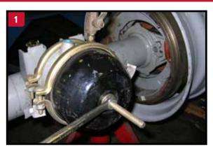
If the axle is equipped with spring brakes, manually cage the brakes following the manufacturer's recommended procedures.
