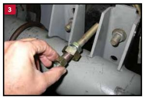
When installing a Gunite slack adjuster with a collar lock clevis, place the 1-1/4" collar nut on the push rod against the 15/16" jam nut. Next thread the  $\frac{3}{2}$ " hex nut onto the push rod.
