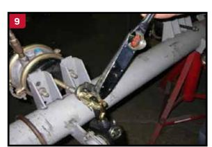
Using a torque wrench, tighten the 1-1/4" collar nut to the clevis using 40 to 50 ft. Ihs of torque
