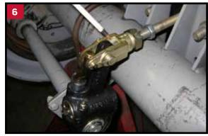
Before attaching the collar nut to the clevis, check to make sure the threaded push rod is fully engaged in the ¾" hex nut. If the push rod does not have full engagement, a new push rod must be installed and cut to length. Refer to the section on cutting a new push rod to length in the Gunite service manual, WE3.001.
