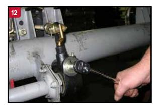
Pre-adjust the brakes by rotating the hex extension clockwise until the brake lining contacts the brake drum. Back the slack adjuster off by rotating the hex counterclockwise ½ turn. Backing off a new slack adjuster will require up to 50 ft. lbs. of torque. A ratcheting sound will be heard when backing the slack off. After completing this step, uncage the spring brake
