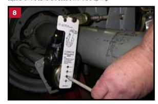
Align the slack by adjusting the %" hex nut on the push rod until the appropriate centering hole on the template aligns with the center hole on the camshaft. The template is provided with centering holes for 5", 5.5", 6", 6.5" slacks.
