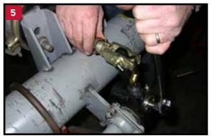
Using the hex extension and a wrench, adjust the slack so that the collar lock and nut aligns with the threaded area of the clevis.
