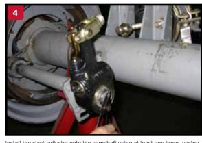
Install the slack adjuster onto the camshaft using at least one inner washer to align the slack adjuster with the brake chamber push rod and enough outer washers to allow no more than 0.060" movement of the slack adjuster on the camshaft. Secure with the snap ring.
