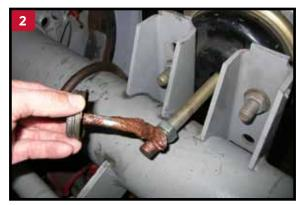
Apply anti-seize to the chamber push rod threads before installing the new clevis. Also apply anti-seize to the camshaft splines at this time.
