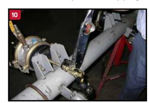
Once the 1-1/4" collar nut has been properly tightened to the clevis, tighten the 15/16" jam nut against the collar lock nut using 40 to 50 ft. lbs. of torque.
